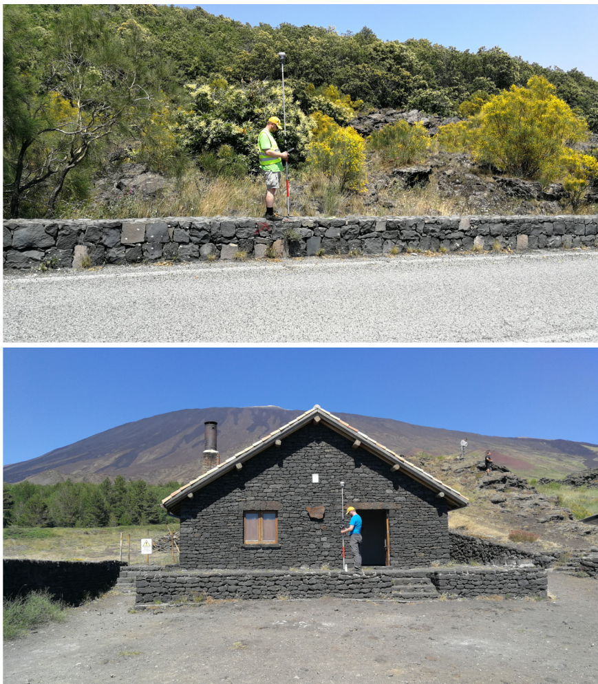
Fig. 5. GNSS measurements on one of relative benchmarks situated on the top of roadside rock-wall (top) and in the front of a refuge with an absolute gravity point inside (bottom).
