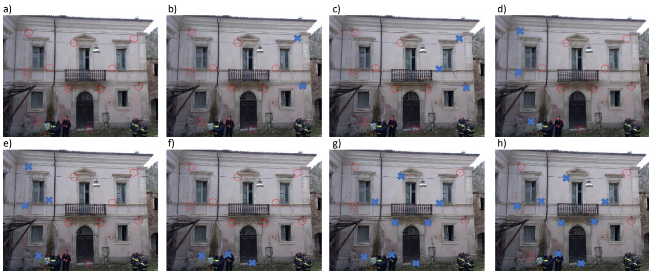
Figure 8. Configurations of measuring point for the house: a) "Ref" (reference); b) "Config 2"; c) "Config 3"; d) "Config 4"; e) "Config 5"; f) "Config 6"; g) "Config 7"; h) "Config 8".
