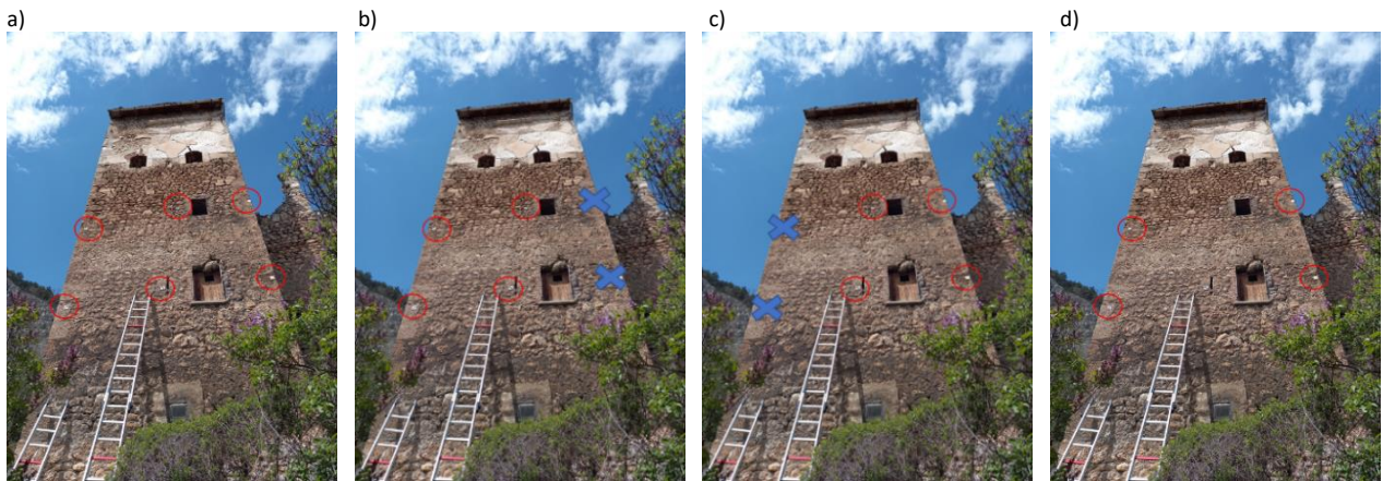
Figure 9. Configurations of measuring point for the tower: a) "Ref" (reference); b) "Config 2"; c) "Config 3"; d) "Config 4".
