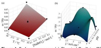
Figure 1. Surfaces responses (a) Chemical Oscillator (BZ reaction) and (b) Electrochemical Oscillator (Cu/Cu<sub>2</sub>O - Cathodic Deposition).
