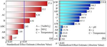
**Figure 2**. Pareto chart representing the significance of the Effects with confidence level of 95 % (p = 0.05) for (a) BZ reaction and (b) Electrochemical Oscillator (Cu/Cu<sub>2</sub>O - Cathodic Deposition).
