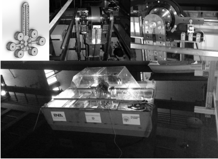
Fig. 6. Pendulum on the left, PTO and PTO frame in the middle, PTO load cell detail on the right and moored device at the INSEAN wave tank on the bottom.
