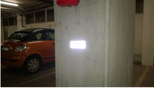
Fig. 9. Reflective marker used for the point-by-point comparison of registrations.
