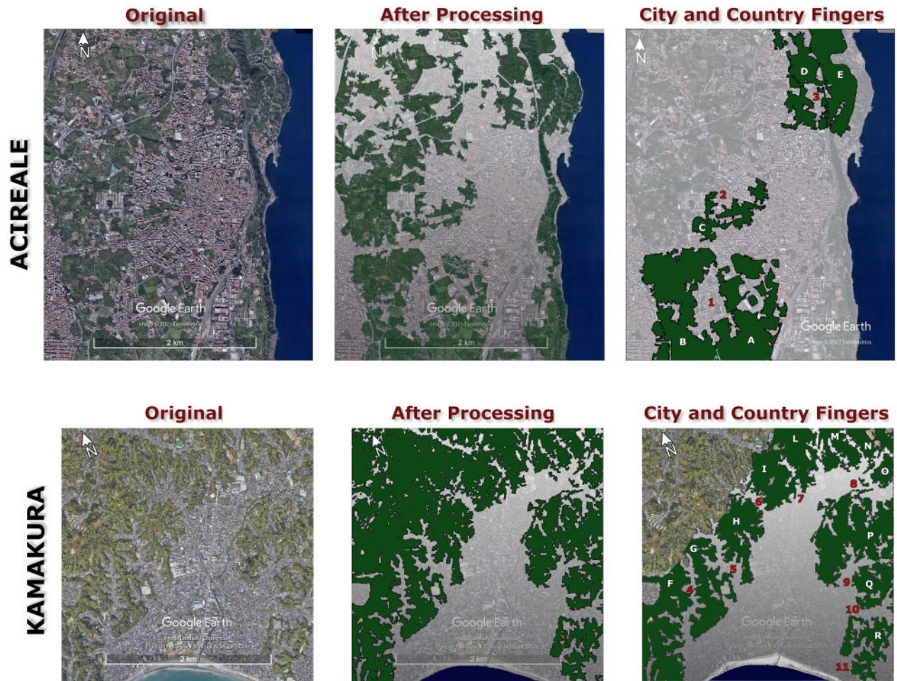
Figure 4: The results of the image processing of the Acireale and Kamakura cities. In the figures on the left the original image, in the central ones the result after the processing phase and in the figures on the right of the country and city fingers for both places indicated by letters and numbers. The vegetation is shown in green and the urban center in transparent gray
