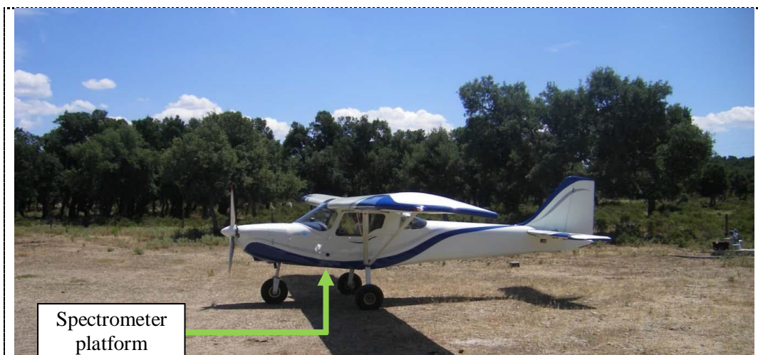
Figure 1. Ultralight airplane employed for the measurement campaign conducted in San Teodoro (Olbia-Tempio - Sardinia) using the spectrometer platform.
