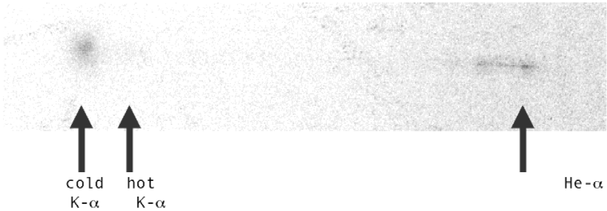
Fig. 4. This film shows the cold K_{\alpha} lines and the He_{\alpha} line; these two lines have been used to get a calibration of the wavelength scale. The shot energy was 4.22 J and the target was 2.2 \mu\text{m} Al foil.
