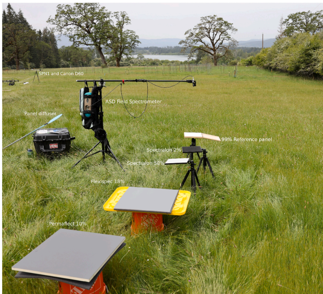
Fig. 2. Example of the reference panel setup at CGOP in support of UAV-HSI acquisition. The tripod with the SPN1 and camera with fisheye lens can be seen in the background. The tripod system used for the ASD spectroradiometer is implemented specifically to avoid operator influences on the measurements and to maintain consistent viewing conditions to mitigate the complications due to the spectral and angular properties of reference panels (Elmer et al., 2020; Soffer, 2014).
