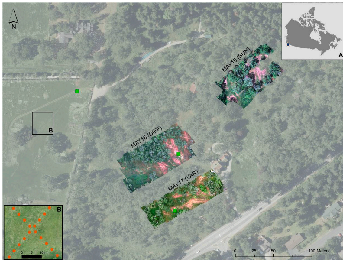
Fig. 1. Meadow section of the Cowichan Garry Oak Preserve (CGOP) with hyperspectral mosaics (true color band combination R: 641 nm, G: 549 nm, B: 461 nm) for imagery acquired May 15–17, 2019. Green squares correspond to the location of reference targets. Inset A shows location of study site in Duncan, British Columbia, Canada. Inset B shows the boresight calibration ground control point setup. (For interpretation of the references to color in this figure legend, the reader is referred to the web version of this article.)
