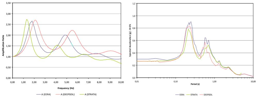
Fig. 4. 1-D results: amplification ratio and response spectra using scaled 1693 seismograms.
