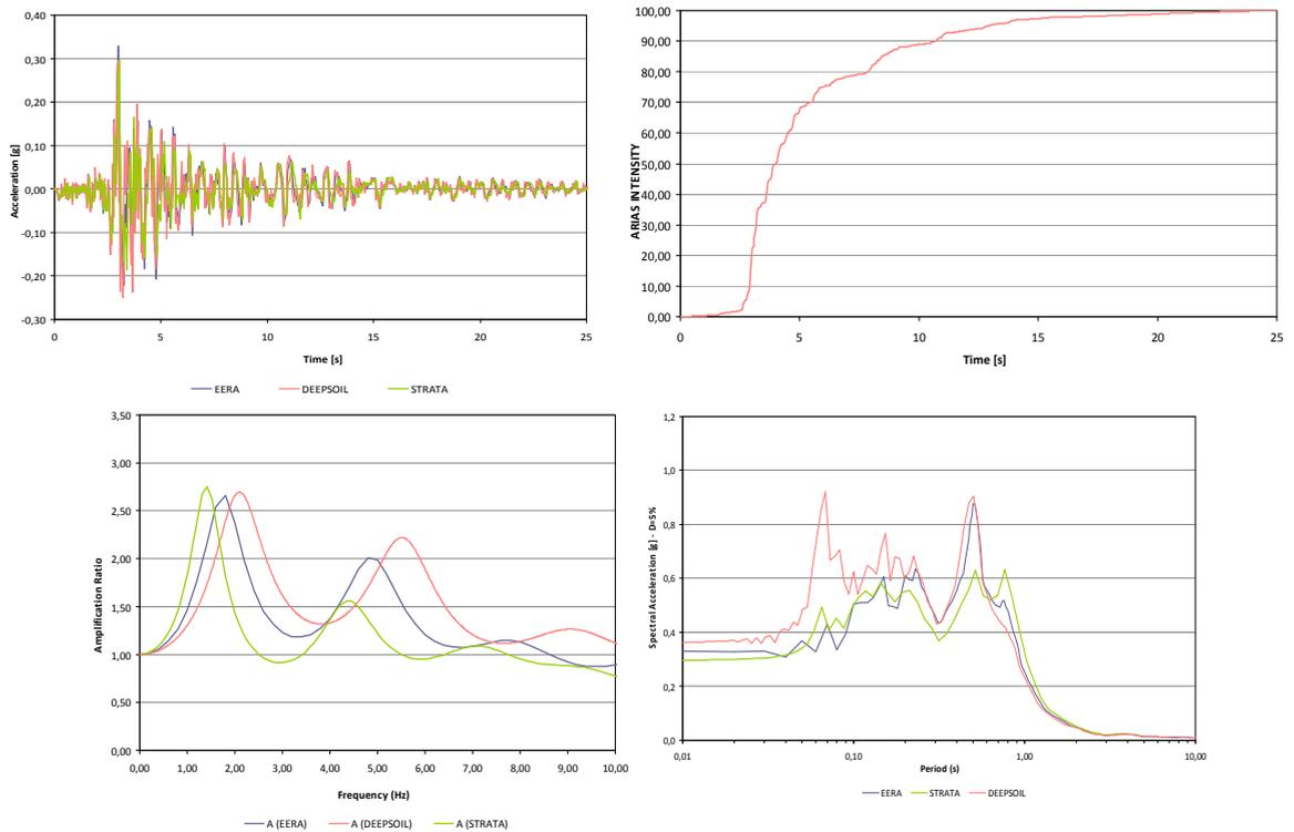
Fig. 5. 1-D results of soil response analysis using as input the scaled 1990 accelerograms in the Sortino recording station.
