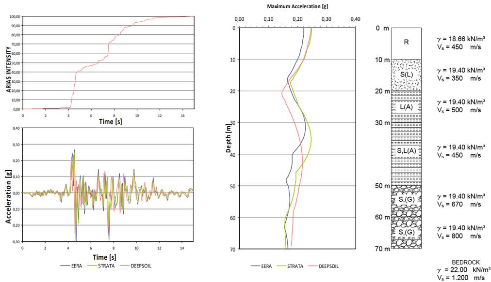
Fig. 3. Maximum accelerations at the surface, maximum acceleration with depth and Arias intensity using scaled 1693 seismograms in the soil column 1. R = fill and debris; S (L) = sands and silts; L (A) = silts and clays; S, L (A) = sands with silts and clays; S (G) = sands and gravels.
