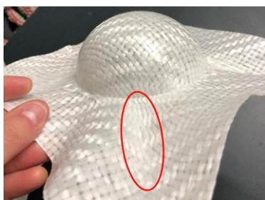
Fig. 8. The shear deformation of the textile in the zone between the springs and the semi-spherical part.
