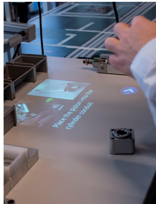
Fig. 5. Participant while assembling with the projection-based system.
