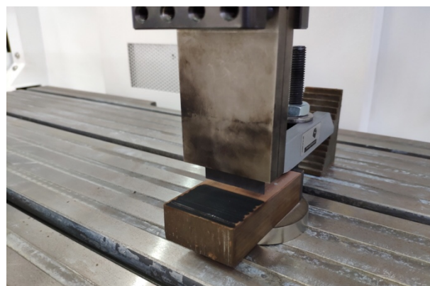
Fig. 2. Copper workpiece setup for tool electrode dressing.
