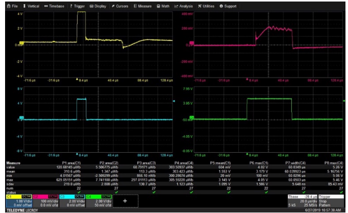
Fig. 17. Appearance of current, voltage and machine control board signals on the oscilloscope screen.
