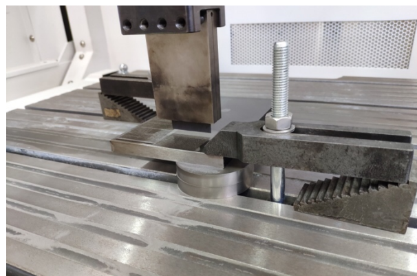
Fig. 1. Steel workpiece and tool electrode setup for the EDM tests.
