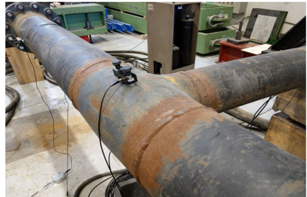
Fig. 19 Green points show acoustic emission signals detected on the Tee joint during the HS tests (left). Tee joint component (right)
