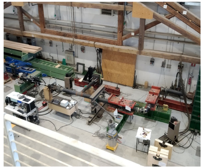
Fig. 10 Experimental setup consisting of the physical substructure and the transfer system
