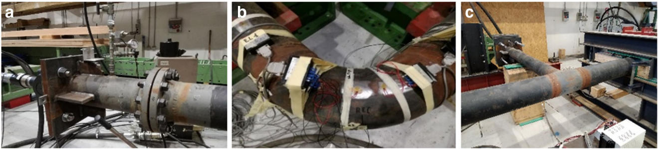
Fig. 11 Close up view of the experimental components. (a) bolted flange joint, (b) piping elbow and (c) Tee joint
