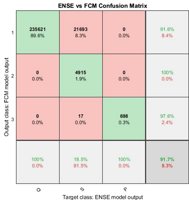
Fig. 30 Confusion Matrix obtained assuming as target the output of the ENSE supervised classifier and as output class the output of the FCM clustering algorithm
