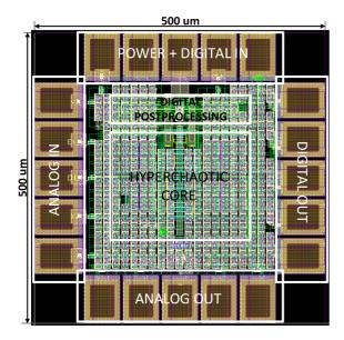
Fig. 15 Layout diagram of the chip
