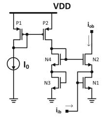
Fig. 6 Circuit design of current square
