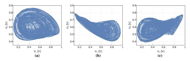
**Fig. 11** Trajectories of the chaotic outputs **a**  $V_1-V_2$ , **b**  $V_1-V_3$ , and **c**  $V_1-V_4$
