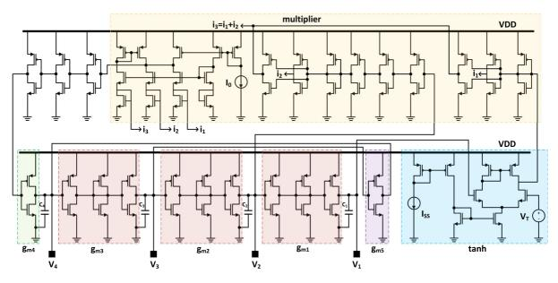
Fig. 9 Circuit design of the proposed 4D hyperchaotic system
