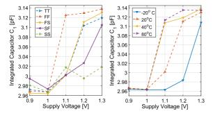
**Fig. 10** Integrated capacitor  $C_1$  according to PVT variations
