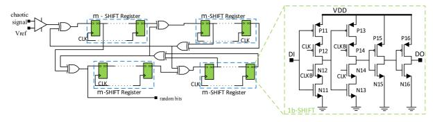
Fig. 14 Circuit design for post-processing based on dynamic D Flip-Flop
