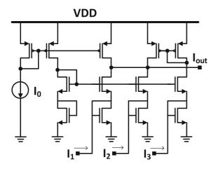
Fig. 8 Multiplier circuit design
