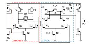
Fig. 13 Comparator circuit design
