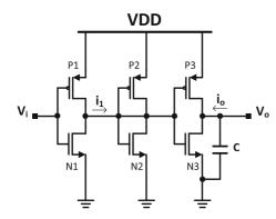
Fig. 5 Integrator circuit design
