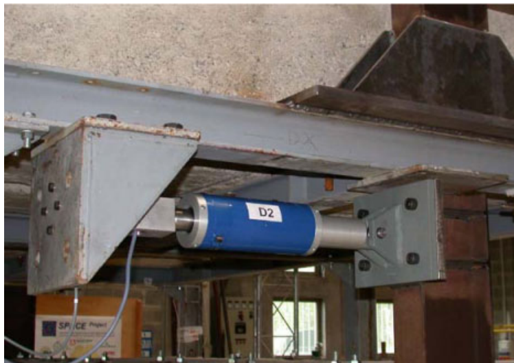
Figure 2. MR damper and detail of connection to the structure.
