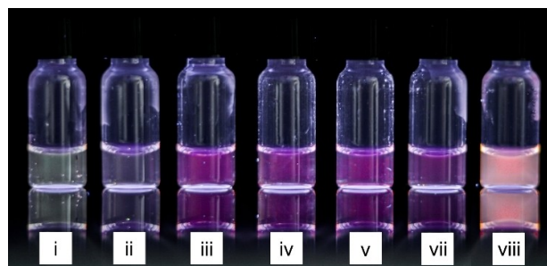
Figure 6. Pictures of the emission color of 3 ( c = 20 \mu\text{M} ) in BPE buffer (i) and in the presence of one equivalent ct DNA (ii), 22AG (iii), a2 (iv), c-kit (v), and c-myc (vi), ty RNA (vii), BSA (viii); \lambda_{\text{ex}} = 366 \text{ nm} .
