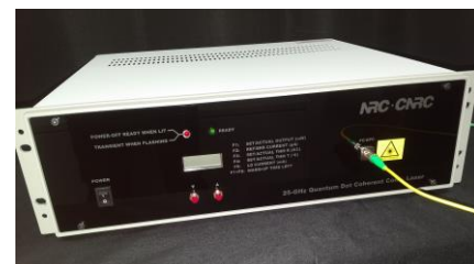
Fig. 8. is a completed rack mount QD C-band 25 GHz CCL module.
