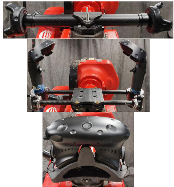
FIGURE 3. Metrology bar, with devices on both ends and its C16 tool mount. Top: A 350 mm long carbon fiber tube, with VLTS's tracker on both ends. Middle: An assembly of two carbon fiber rods and rack, with VLTS's controller on both ends. Bottom: HMD mounted on the end-effector of C16.
