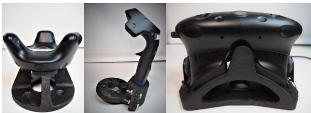
FIGURE 2. Vive tracking devices with their 3D printed mounts for flange ISO9409-1-A63. From left: tracker, Controller, and HMD.
