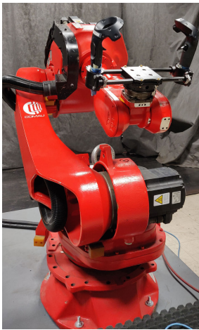
FIGURE 1. Ground truth system: Comau NS16 1.65 foundry hand robot with the mount for controller dynamic analysis attached to the end-effector.
