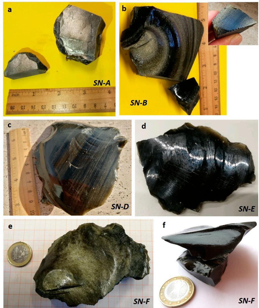
Figure 2. Macroscopic aspect of analyzed samples. (a) Sample SN-A. Note the flat surface, the green color, and the homogeneous, “metallic” hue. The microscopic observations and microanalyses were conducted on the upper surface of the smaller fragment. (b) Sample SN-B showing alternating dark and light bands with different roughness. In the inset, the small fragment used for microscopic observation and microanalysis. (c) Sample SN-D, smooth and with thin bands of different colors. (d) Sample SN-E. Note the absence of hue and the green color, visible only on the thinner edges. (e) Sample SN-F, homogeneously green with changing golden hue. Microscopic observations and microanalyses conducted on the upper surface. (f) Sample SN-F. Surface artificially hammered, roughly orthogonal to the surface shown in Figure 2e. Note the different, darker color.
