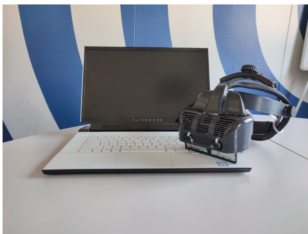
FIGURE 1. The laptop running the computing unity and the custom-made hybrid optical/video see-through head-mounted display.
