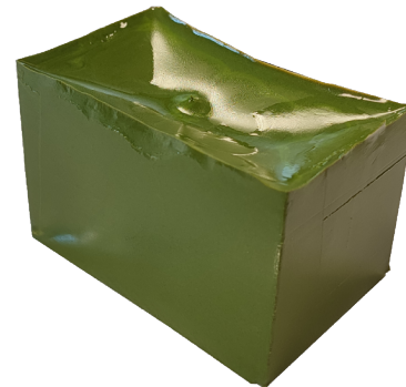
(a) PVC-P phantom doped with graphite and dyed in green.
