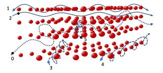
**Figure 3.** Various channeling regimes for positively and negatively charged particles in crystals. 0—amorphous orientation; 1—planar orientation for a negative charge; 2—planar orientation for a positive charge; 3 and 4—axial orientation for a negative charge; and 5—axial orientation for a positive charge.
