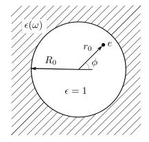
**Figure 8.** Scheme of a cylindric cavity of radius  $R_0$  in the infinite dielectric, characterised by the permittivity  $\epsilon(\omega)$ , with a particle of the charge *e* moving inside the cavity. For the cavity, we choose  $\epsilon = 1$ .
