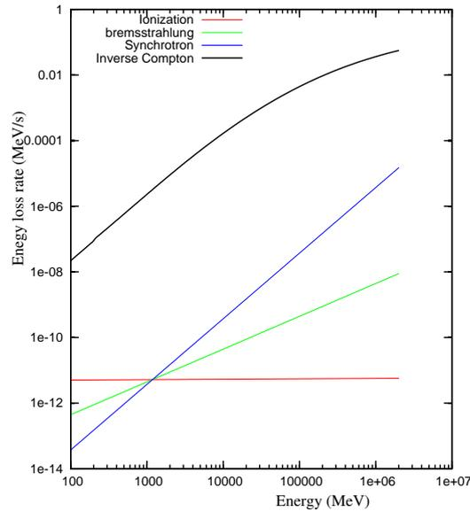
Fig. 2. Energy loss rate of electrons inside the heliosphere at 1 AU, which is due to several processes.
