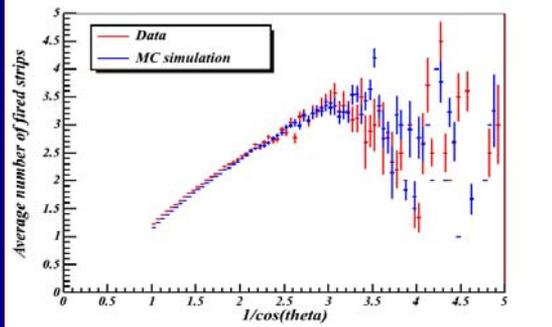
Fig. 6. Hit strip multiplicity vs  $1/\cos\theta$  and MC comparison
