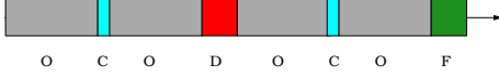
Fig. 1. Structure of the cell : O, C, F, D drift, RF cavity, focusing , defocusing quadrupole
