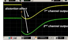
Output signal of two different preamplifier channels operated at 77K and connected to the outside through 12-m RG168 cables: when one common power supply is used, and a considerable power has to be delivered, the output exponential signal shape is distorted by the bounce effect on the common power supply. An appropriate separation of the input/output stages power supplies is mandatory to eliminate the distortion.
