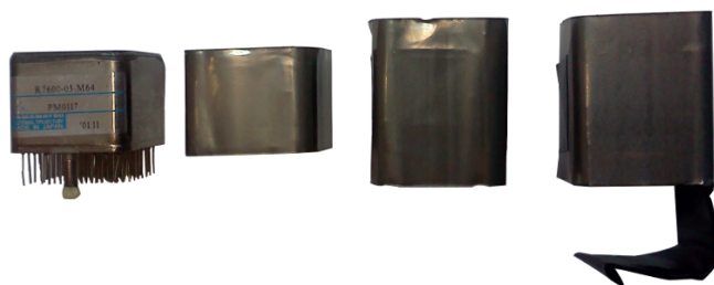
Figure 8. The R7600 Ma-PMT and the three magnetic shields that were tested.
