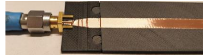
Fig. 1. A photograph of the test assembly for the proposed technique. A puzzle-like launcher (black material) is used at each end as an intermediate element between the end-inserted coaxial connector and microstrip line on the substrate-under-test (gray material). Launchers are then de-embedded to provide measured S-parameters referenced at the test material edges.
