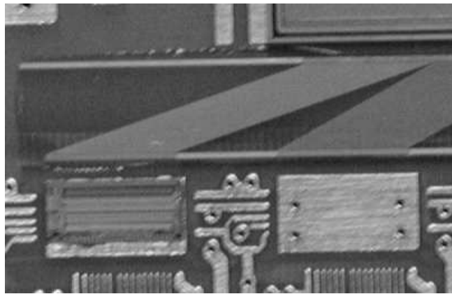
FIGURE 3. Detail of the pitch adapter which connects the detector (top) to each of the 6 RX64 ASICs (bottom).
