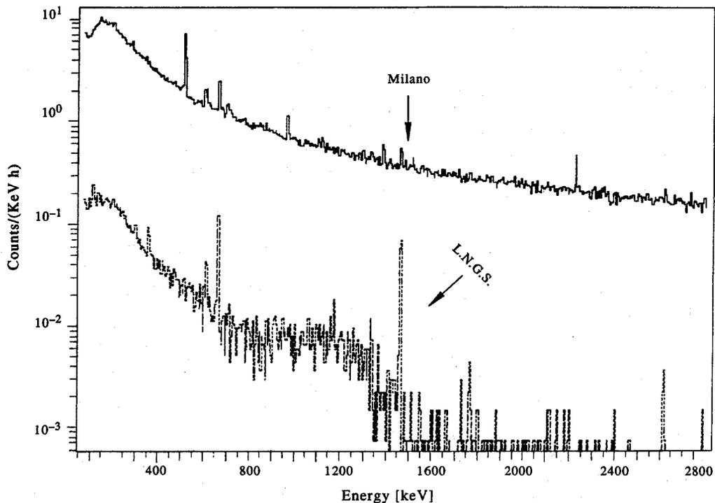
Fig. 1. Background gamma spectra with Ge detector obtained in Milano and LNGS with proper shielding.
