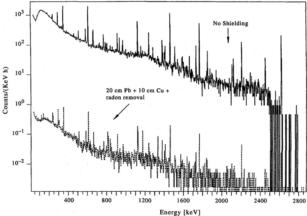
Fig. 3. Background gamma spectra with a GeHP detector in air and with proper shielding.
