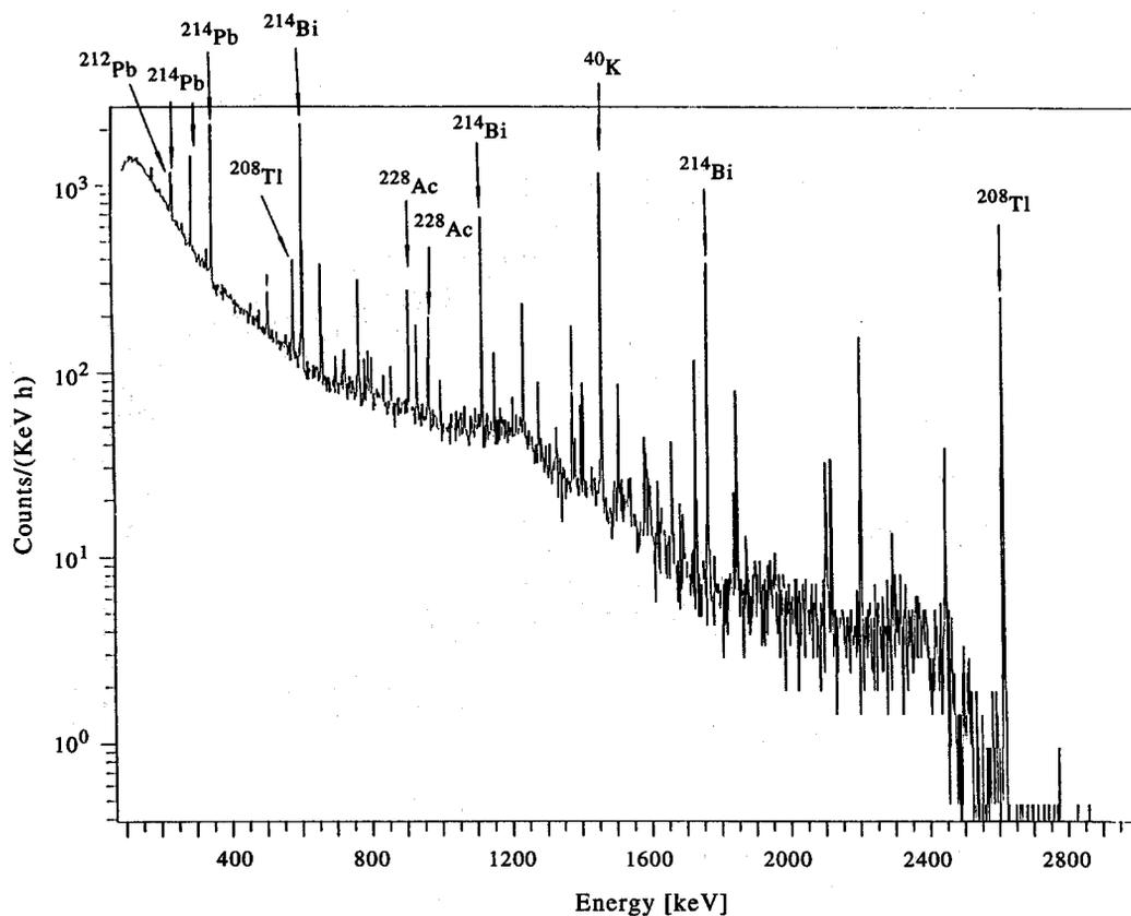
Fig. 2. Gamma energy spectrum from natural environmental radioactivity measured with a GeHP detector in hall C at LNGS.
