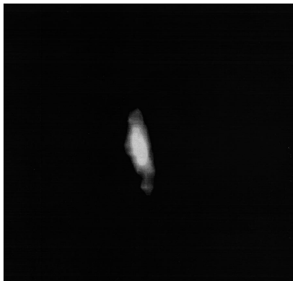
Fig. 7. Beam image at 2 GeV. The scale of the figure is 100 \times 100 pixels (in horizontal direction 1 \text{ px} = 0.097 \text{ mm} and in the vertical direction 1 \text{ px} = 0.064 \text{ mm} ; the different ratios are due to the frame grabber acquisition).
