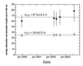
Figure 1. Values of the absorption and attenuation lengths at 440 nm measured during five different campaigns. The reported values are the average in the depth region 2850-3250 m. Dashed lines are the average over the five campaigns.
