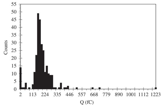
Fig. 8. Minimum Ionising Particle spectrum for  $V_b = 250$  V.
