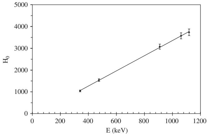
Fig. 4. Linearity of the detector response.  $H_0$  is the centroid of the photopeak.
