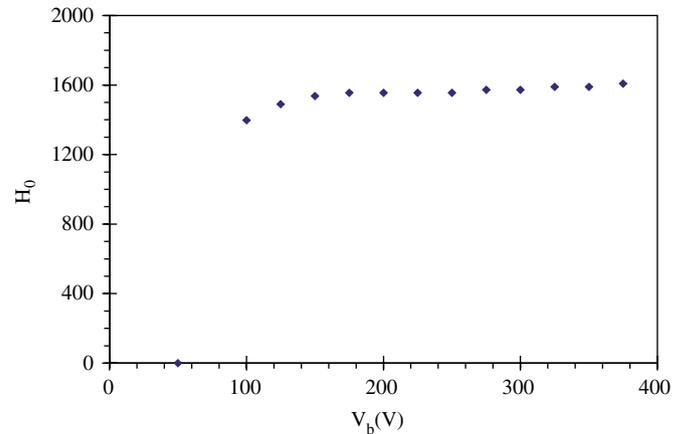
Fig. 6. Compton edge position versus bias voltage at 4.7 K.  $H_0$  is the centroid of the photopeak.
