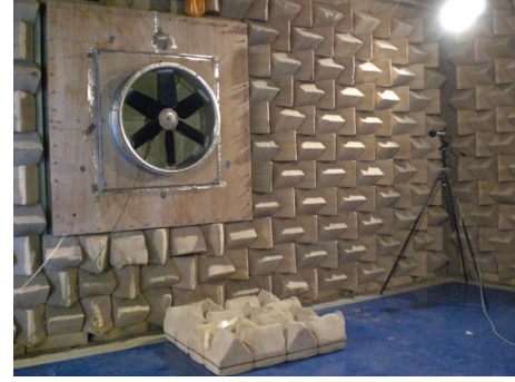
FIGURE 2: Test rig set-up in the semianechoic room.
