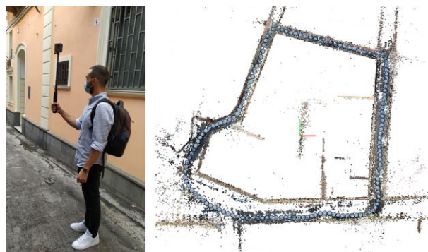
Figure 4. On the left: GOPRO Fusion 360 on site during acquisition. On the right: sparse cloud with points of acquisition inside Metashape.
