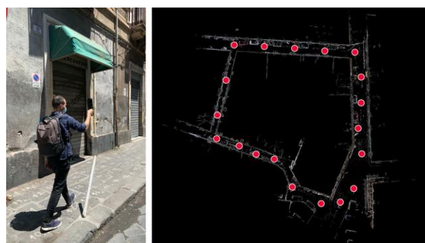
Figure 5. On the left: BLK2GO on site during acquisition. On the right: imported point cloud in Register360.
