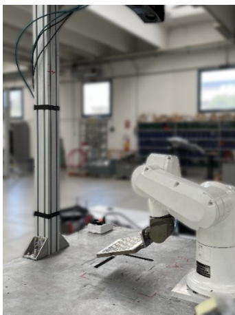
Figure 4. Robotic setup used for the calibration of the O3DCMS. The same 3D poses of the calibration board were used while calibrating both devices to grant repeatability.
