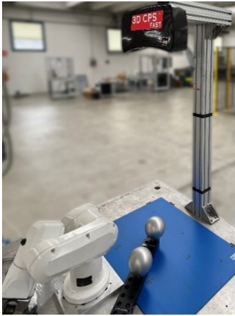
Figure 3. Setup used during the execution of the tests on the 3DCPS Fast scanner. The device, the robot used for the calibration, and the ball-bar artifact are shown.
