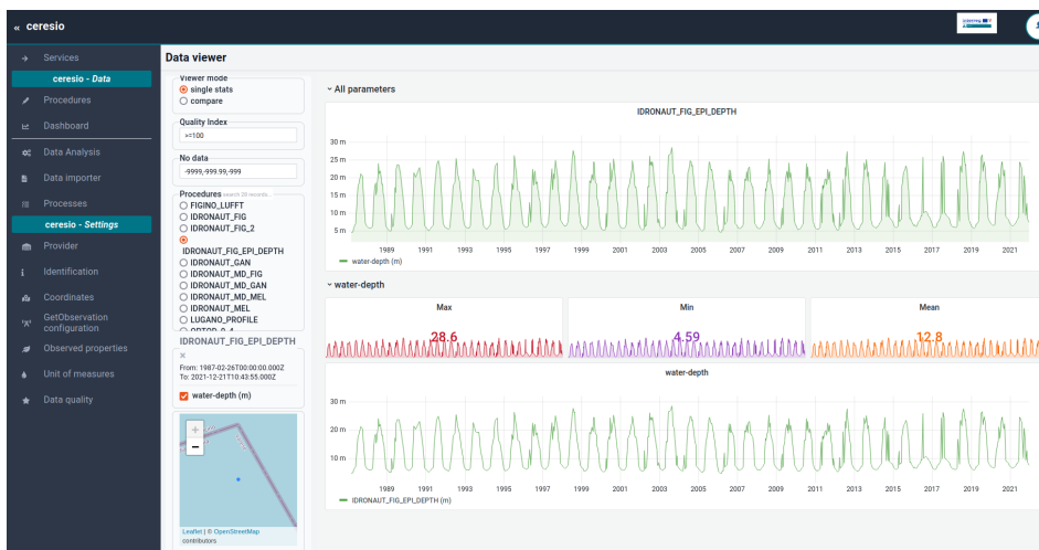
Figure 8. Epilimnion depth calculated using the LakeAnalyzer web plugin and the monthly data collected by the traditional campaigns, previously standardized and imported into istSOS.
