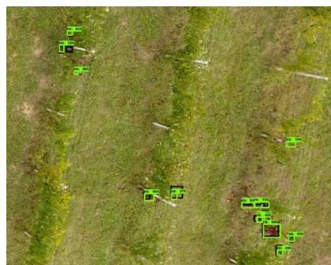
Figure 10. Object detection test results with the Faster RCNN_ResNet 101 architecture (test 4) on different types of images. In black, the reference data and in green the bounding box detected and the confidence score.
