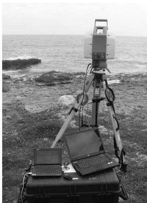
Fig. 10. The terrestrial laser scanner (TLS) Leica Scan Station 2 at work.
