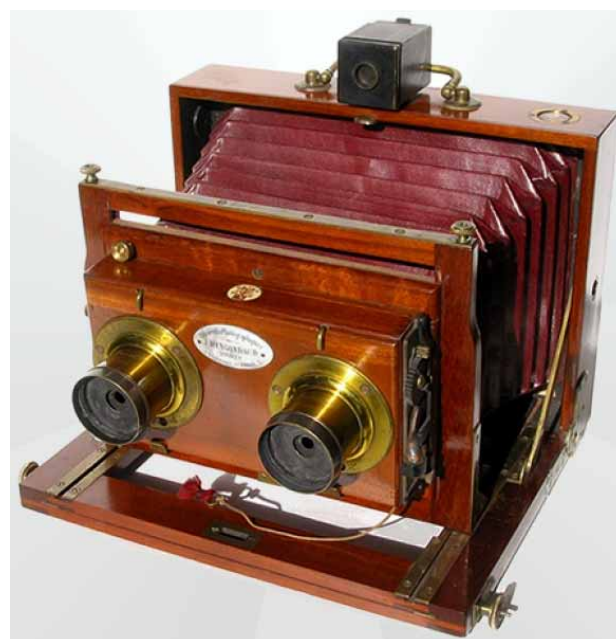
Figure 6. Double lens camera for stereoscopic photographs, Reygondaud model, 1890.
