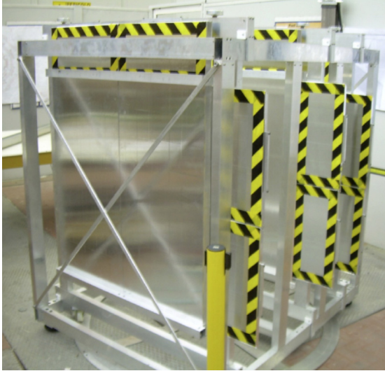
Figure 3. The detector frame with the three X-Y planes mounted. The frame can be oriented using the rotating platform visible at the bottom.
