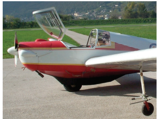
Fig. 3. A close look at the sensors outside the motorglider on the left undercarriage leg.
