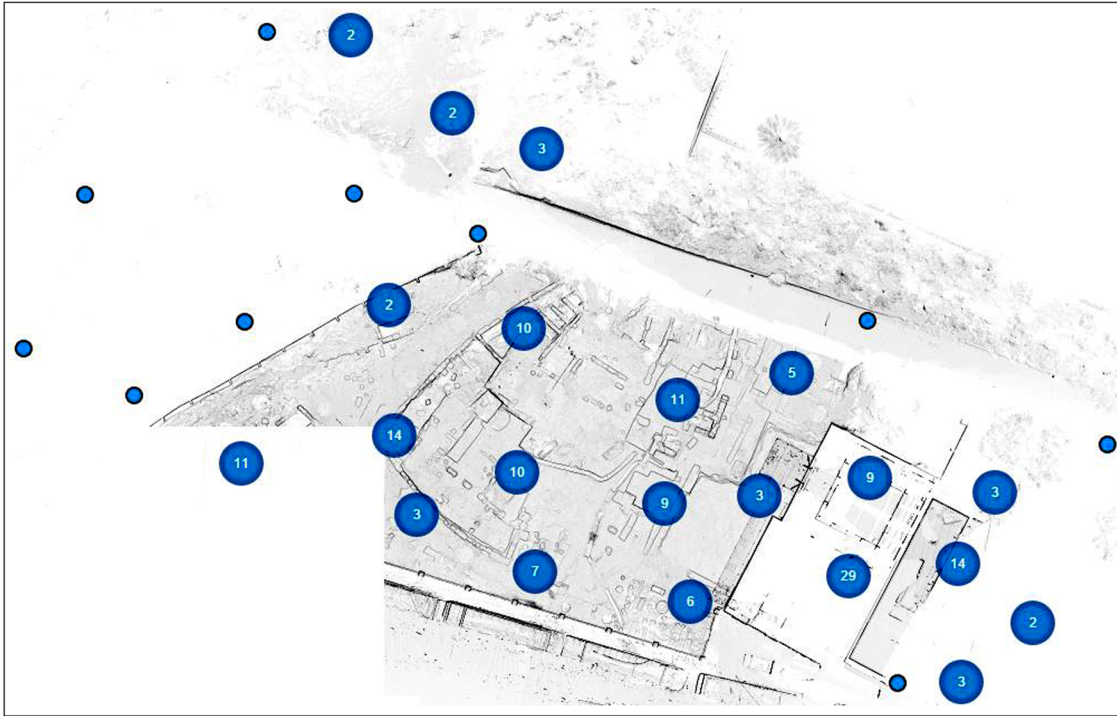
Figure 13: Plan of the Domus Romana with indication of the 3D scanning stations.
