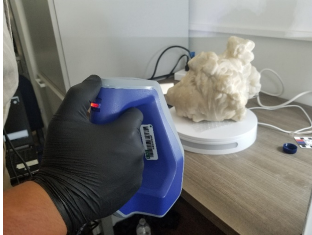
Figure 28: Artec Space Spider structured light 3D scanning station at the Domus Romana museum in Rabat, Malta.
