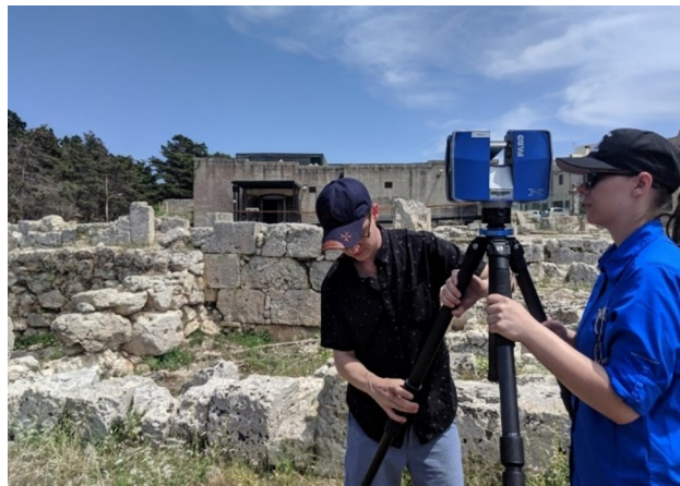
Figure 9: 3D capturing with Focus ×330 laser scanners of the external area of the Domus.
