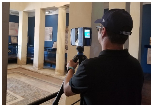
Figure 10: 3D capturing with Focus ×330 laser scanners of the interior of the Domus.
