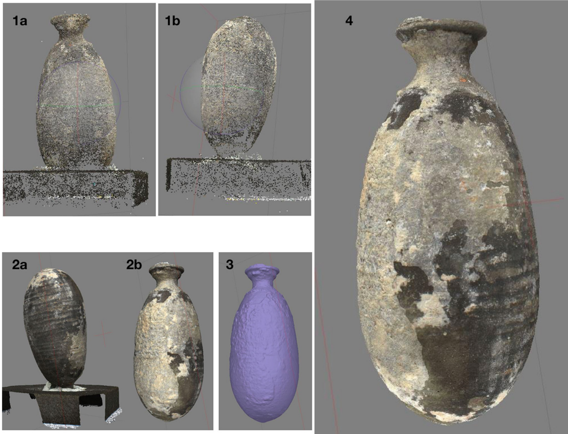
Figure 35: Digital photogrammetry processing steps in Agisoft Metashape: (1a and 1b) sparse cloud resulting from the align images function, with two different chunks processed for the two artefact positions; (2a) dense cloud of the chunk featured in 1b; (2b) aligned dense clouds from the two chunks with support material manually removed; (3) untextured mesh from the build mesh process; and (4) final textured mesh (Kingsland, 2019).
