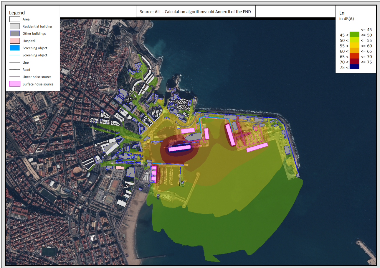
Figure A5: GNM of Melilla port area considering all the noise sources using the algorithms of the old Annex II of the END. L_{night} indicator
