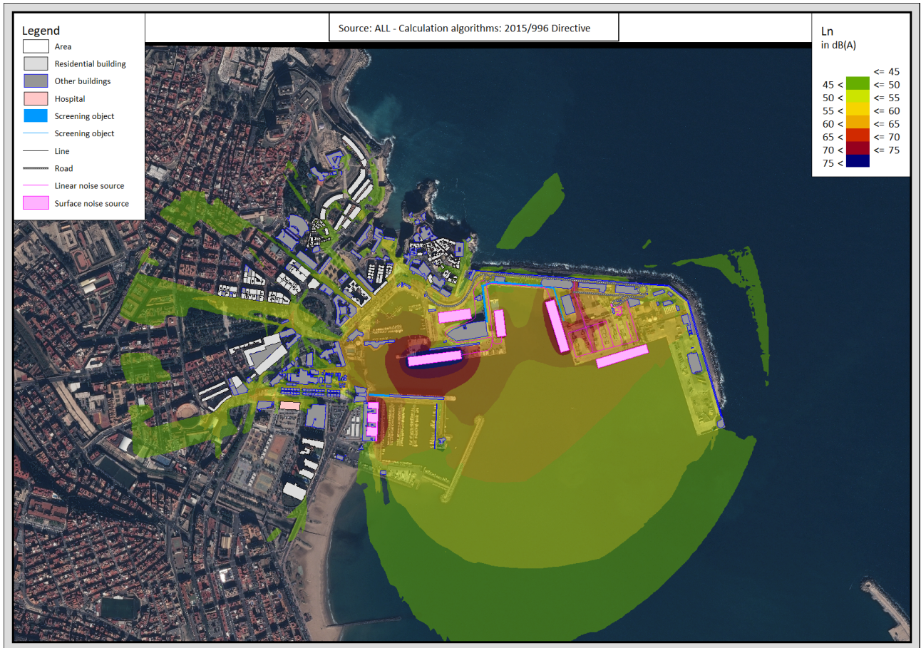
Figure A4: GNM of Melilla port area considering all the noise sources using the algorithms of the 2015/996 Directive, L_{night} indicator
