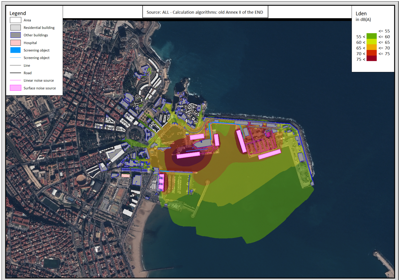
Figure A2: GNM of Melilla port area considering all the noise sources using the algorithms of the old Annex II of the END. L_{den} indicator
