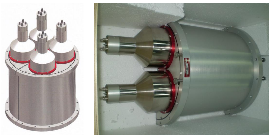
Fig. 6. Left panel: A drawing of the 14x14 inch segmented NaI detector of the Tandem Accelerator Laboratory. Right panel: A photo of one of the two segments of the detector.
