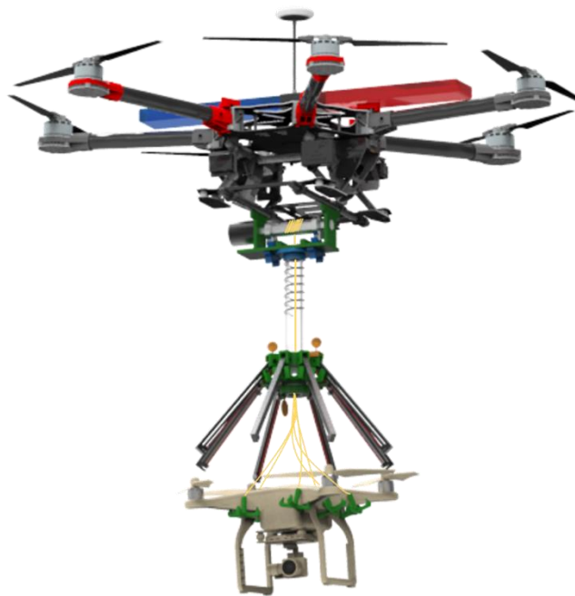
FIGURE 1. Conceptual design of the deployable hook retrieval system (DHRS);
