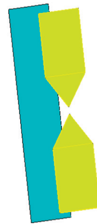
Figure 1. Two-element Yagi-Uda antenna immersed in water, operating at 434 MHz
