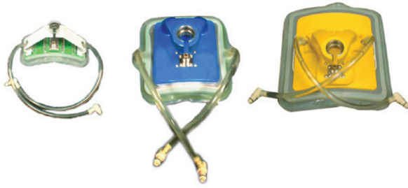
Figure 1. CCMA applicators: from left to right the \alpha , \beta and \gamma applicators.
