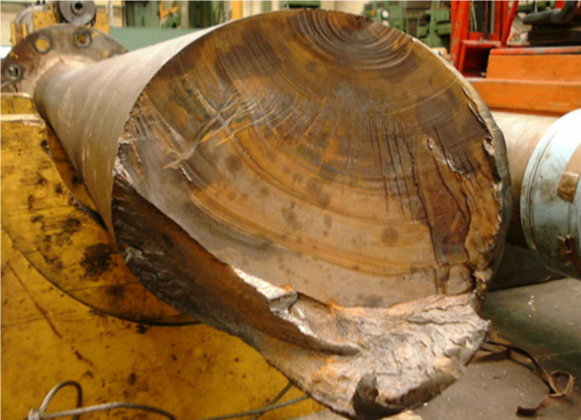
Figure 5 Fractured propeller shaft
